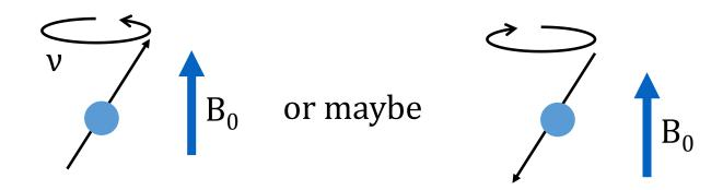
$B_0$  is applied field  $\nu$  speed of rotation (many MHz /  $10^6$  Hz)
